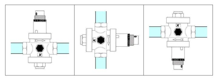
Pressure reducing valves can be damaged by dirty water; therefore we advise to install a self-cleaning filter upstream before the pressure reducer, in order to protect the valve and any other mechanism (thermostatic mixers, taps, etc.).
