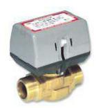
2-Way Motorized Zone Valve for SPDT (3 wires) or SPST (2 wires + common). The 2-way valves VC6613A / VC4613A are used for temperature control, in conjunction with thermostats, in zone heating systems. They are also used in fan-coils installations with 2 or 4 tubes.
