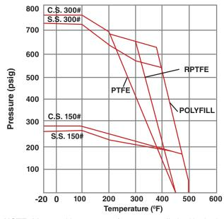
**NOTE:** Max. working pressure/temperature limited by both flange rating, seat and body seal capability.
